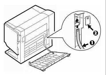
6. Place the large stopper over the tab on the cover and turn it to lock it in position.
